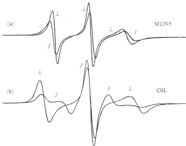
Fig. 4 ESR spectra of spin probes in S_A phase.
